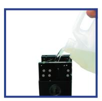
Lower Transport Modules carefully into their respective tanks. Top up - the correct liquid level will show half way up the sight glass.
