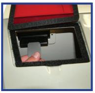
Put hands through Loading Gloves and strip wrapping from film, insert film into Entry Slot. Touch the Film Entry Slot to initiate processing. A bleep will indicate film detected.
