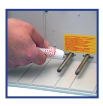
Grease immersion heaters for developer and fixer tanks with the lubricant provided.
