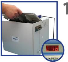
Bring the Lid to the upright position. When operating, indication of the opened lid is displayed as: "Lid". Unscrew the retaining screw at the back of the machine above the plug and lift the Display Panel.
