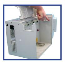
Secure Loader with the two retaining screws. Return side panels and lid panel.
