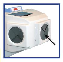
Put hands through loading ports and place film inside Daylight Loader.
