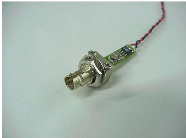
FIG-6.2 – AIMING LASER DIODE ASSEMBLY
