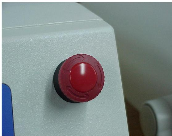
**FIG – 18 EMERGENCY STOP SWITCH**
