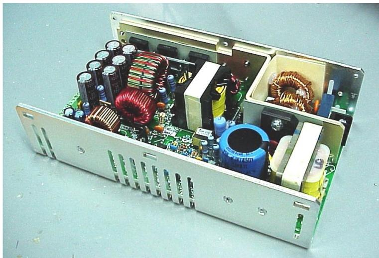
**FIG – 10 AC/DC POWER SUPPLY**
