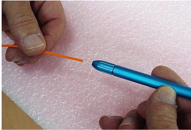
**FIG 26.5- INSERT STRIPPED FIBER INTO HAND PIECE**
