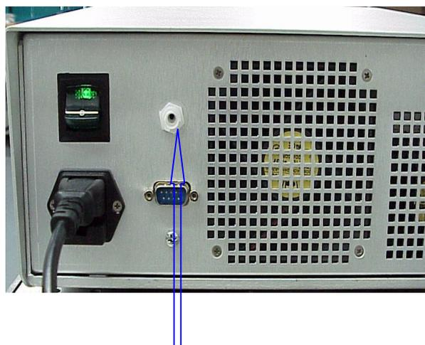
**FIG – 4 FOOT SWITCH CONNECTING**
